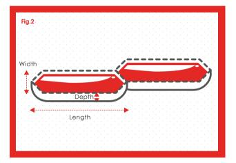
The quality of the lay is far improved by the increased line counts utilised by HVP. The increased amount of cells in a sq/cm create greater resolution in print as the ink releases from the cells in a more controlled manner leading to less reticulation and an improved all over lay. This control element produced by the increased line count enables our customers to print fine vignettes and intermediate areas without large deposits of ink bridging and filling-in.
